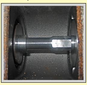
5. Driven disc will bottom out on the chamfer at the end of the axle tube, ensuring accurate installed depth of new seal.
