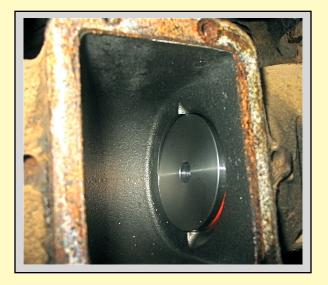
4. Set forcing screw & drive disc in place, rotating screw as needed to press seal into the axle tube.
